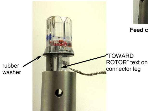
Install connector with "TOWARD ROTOR" text pointing to the rotor.
