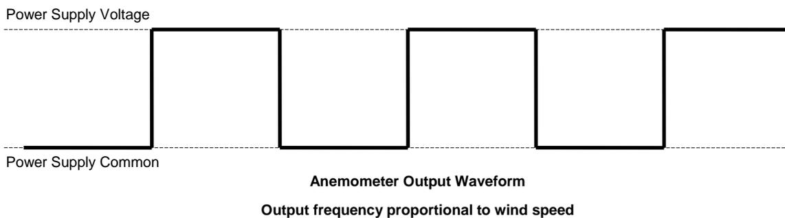
Under normal operation, the frequency varies from 0 Hz to 141 Hz or higher. The anemometer output signal can be timed on either the rising or the falling edges. For best accuracy, time and count many cycles then divide the count by the time for an average frequency. This technique also effectively filters out short-term wind speed variations.
