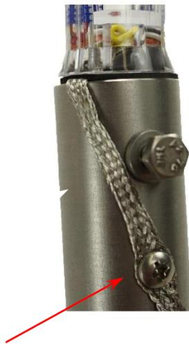
**Suggested method for attaching shield to mast.**
