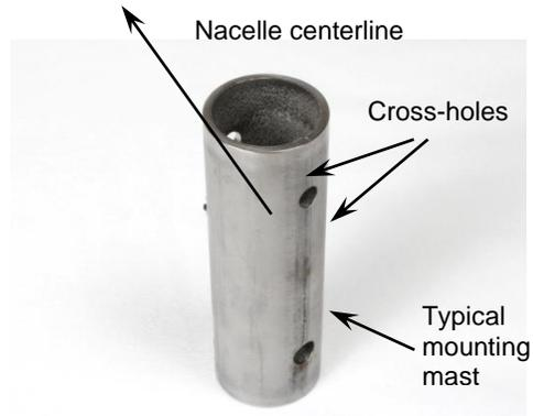
**Align cross-holes parallel to nacelle centerline.**
