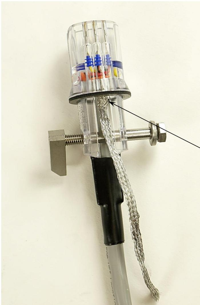
**IF cutting shield wire, cut close to connector base as shown.**
