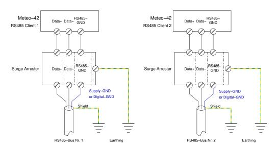
Example: Connection of client interfaces 1 and 2 to RS-485 bus 1 and 2
