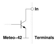
Recommended wiring for a modem with a power control switch
