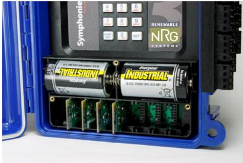
SCM cards installed under battery cover
