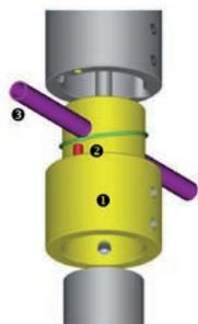
We recommend installing a North ring adapter (1; yellow), which assists aligning the sensor correctly and avoids re-alignment after sensor replacement.
