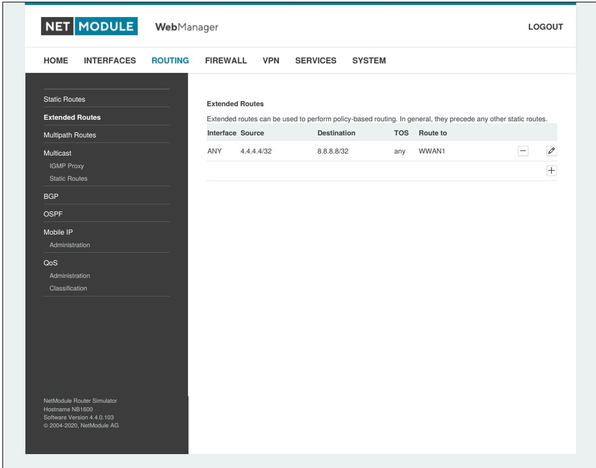
Figure 5.21.: Extended Routing
