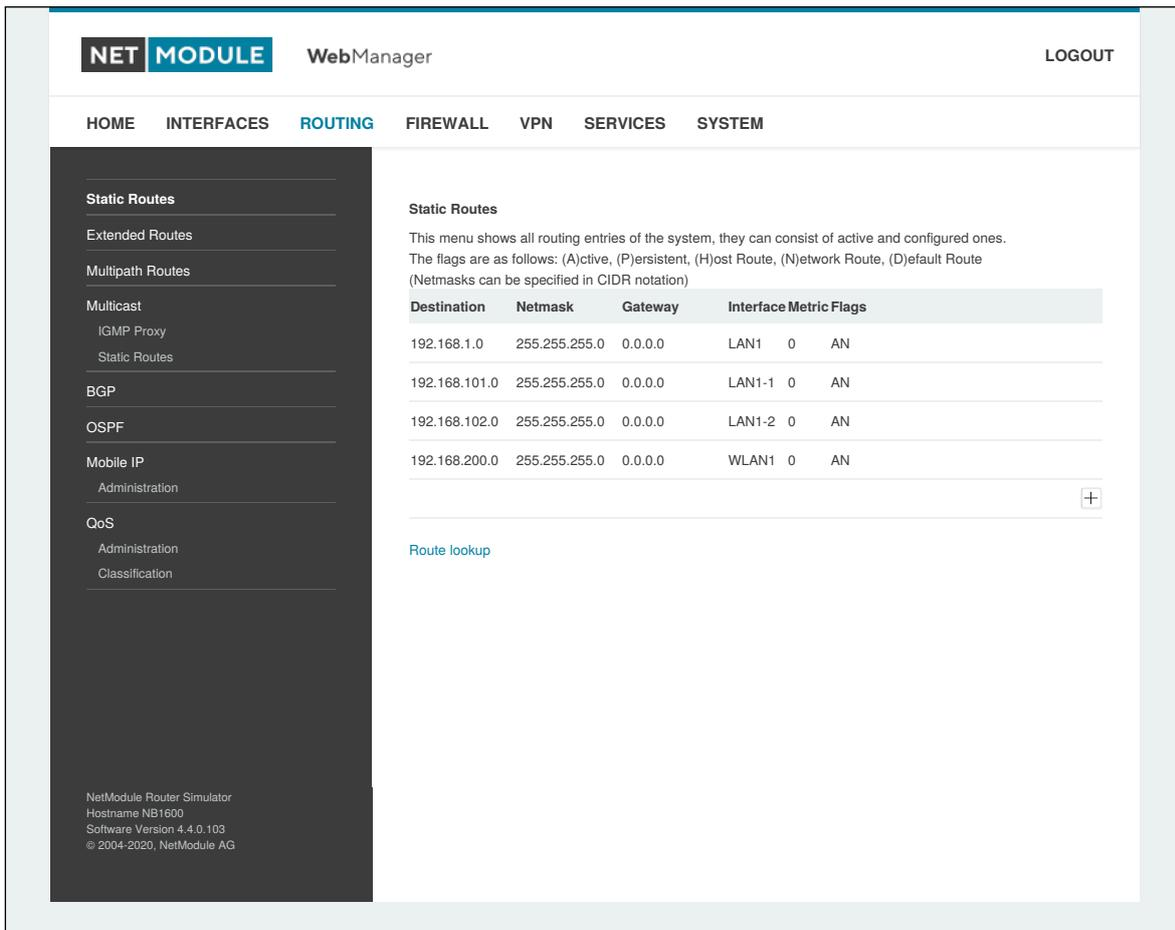
Figure 5.20.: Static Routing
