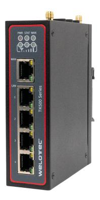
Robust industrial router designed for demanding environments, providing reliable connectivity and integrated cybersecurity features. Five Ethernet Ports, RS-232, RS-485 DIN-Rail mounting and 9 to 36 V DC power supply Integrated Firewall, OpenVPN and IPsec Very compact and rugged housing Fully integrated with Welotec Smart EMS and VPN Security Suite 5 year warranty
