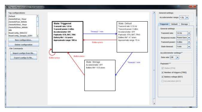
This window enables you to create Quuppa state machine configurations that will be used to set up tags.
