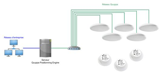
Antennas are positioned in a mesh layout, which can be more or less spread out depending on the desired localization accuracy (i.e. only presence detection, zoning, precise location).
