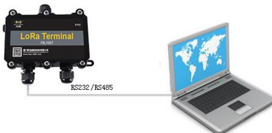
Figure 2-1 Configure connection between F8L10ST and PC
