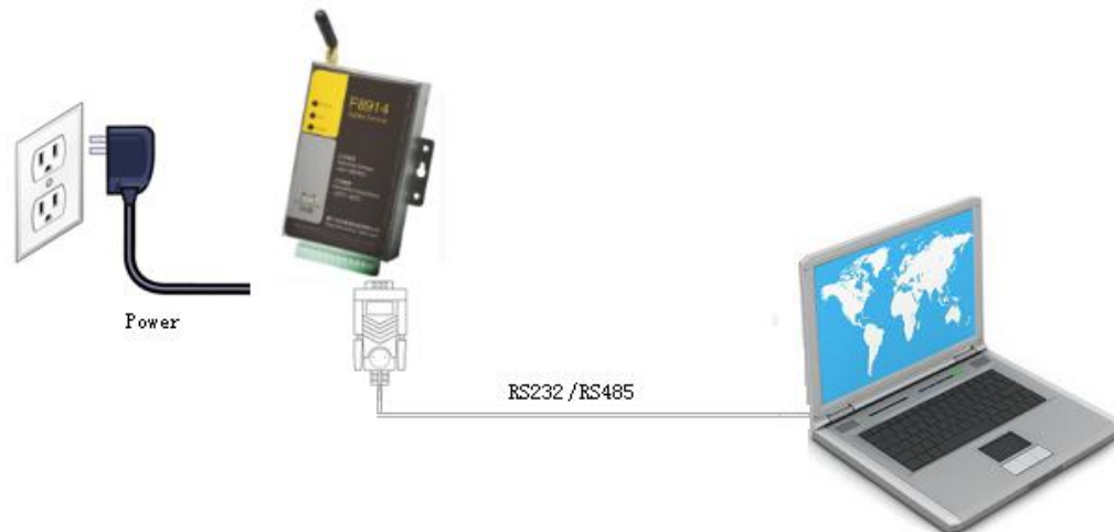
Figure 3-1 F8L10T configuration connection with PC
