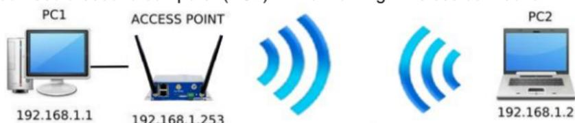
Set up the PC2 Wireless network interface according to the default parameters of the ACKSYS AP device (802.11gn, SSID "acksys", no security).
