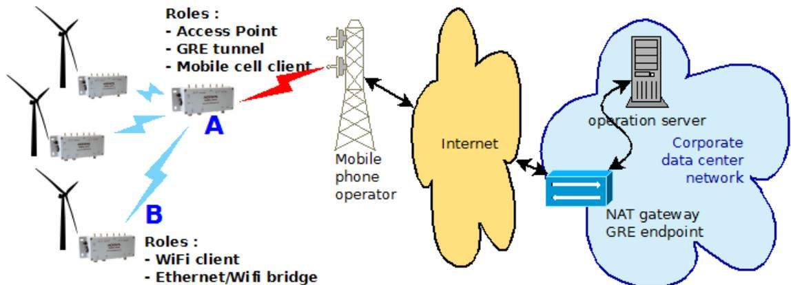
Only the configuration of product 'A' (the plant gateway) is given below. Product 'B' and the operation server share a virtual LAN in the same IP range (192.168.0.0/24), products 'B' being fed their address through DHCP in the range 192.168.0.100... 192.168.0.249. The operation server should have an address such as 192.168.0.1.
