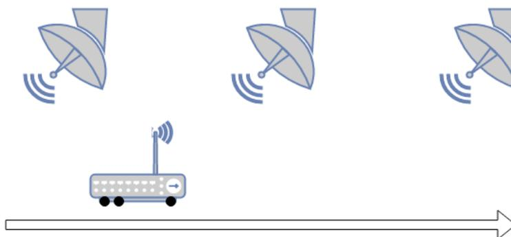
The idea is to reject APs whose signal level decreases. They are supposed to be passed by the vehicle. More precisely, PLH rejects APs whose signal level is lower than one of the preceding values, without time limit as long as the AP remains visible.
