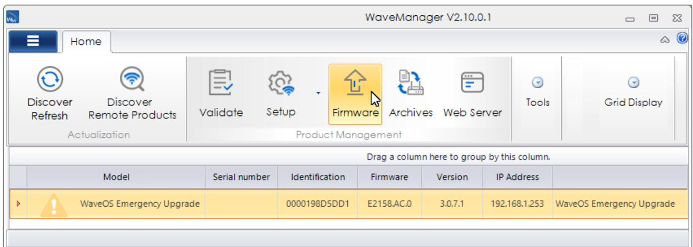
While the product is in **Emergency upgrade** mode it still allows to restore factory settings by pressing the reset button more than two seconds.
