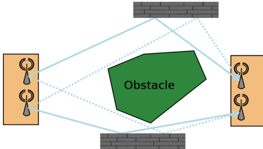
802.11n/ac uses these bounces to allow several independent streams (2 to 4) to be sent and identified simultaneously. At the beginning of the transmission, a well-known pattern is sent. The receiver uses that pattern to calibrate itself and characterize the transmission channel for each antenna.
