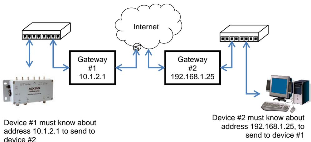
When several routers are available on a single LAN to access various remote LANs, the network devices on the LAN should know about each router’s own address and the remote network addresses they lead to. Usually, one of the routers is designated as “default”, the other ones are treated as exceptions to this default route.
