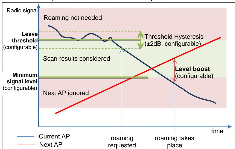
NOTE: the threshold hysteresis is configurable in versions 2.2.7 and later. The “leave threshold” is called “minimum level” in earlier firmwares.
