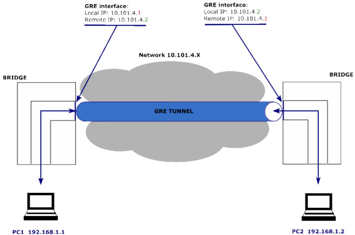
**Layer 2 tunneling over GRE can be configured with the VIRTUAL INTERFACES/L2 TUNNELS.**
