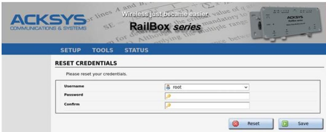
NOTE: We lock and unlock **SSH** accounts after reaching a certain failed number of login attempts with `unlock_time=1200` seconds to respect the standard 62443.
