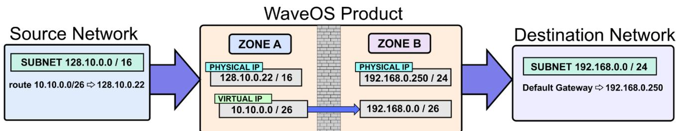
Now if we want to add access to the whole 192.168.1.0 subnet and reach a unique 192.168.2.0 subnet address, we just need to add the virtual addresses and define the proper translation rules. However, it will be necessary to create on the destination interface an alias of the IP address of the product for each of the subnets, in order to be able to define the return path, via static routes, or default gateways.
