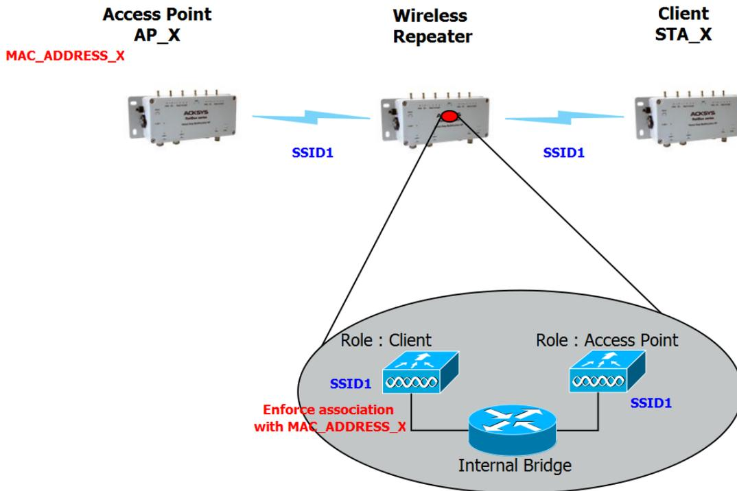
➔ Set a different SSID on client role and Access point role of the repeater.
