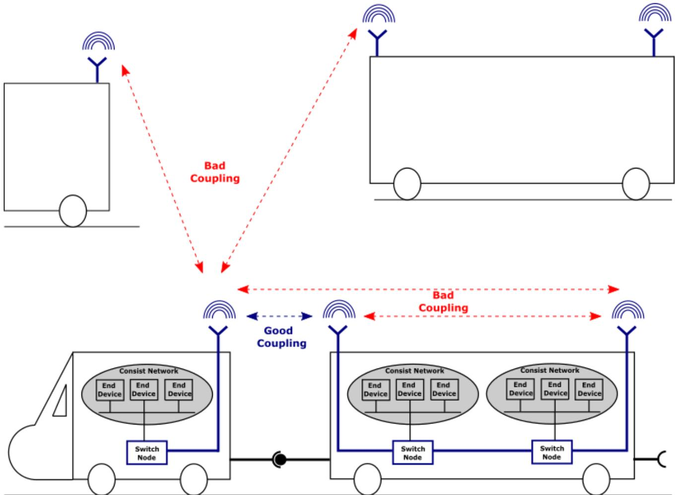
In order to avoid bad coupling, we have to make sure that each switch node only receives signal from the closest valid switch node.
