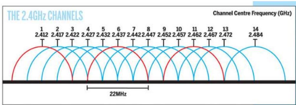
Although the use of “non-overlapping” channels 1, 6, and 11 has limits when products are too close, the 1–6–11 guideline has merit. If transmitter channels are chosen closer than channels 1, 6 and 11 (for example, 1, 4, 7 and 10), overlap between the channels may cause unacceptable degradation of signal quality and throughput.
