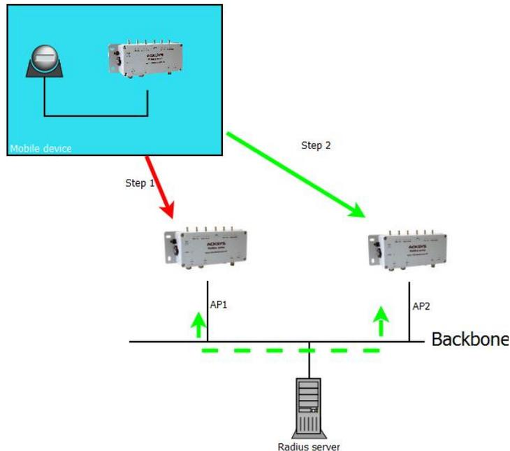
**Step 1:** The Wi-Fi client does a full authentication with AP1. AP1 stores the PMK and temporally keys. This full authentication process produces data that will be stored by the Wi-Fi client for the next step.
