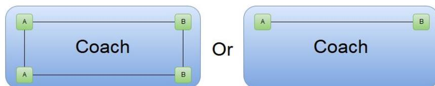
In case of Redundant Mixed Mode, the *Coach end* type becomes irrelevant. In this mode, the inter-carriage Ethernet link provides a way to discover all the devices of the train in one time. At the end of the topology discovery each product will have a list of all devices of the train. Knowing products of his own train allows SRCC to exclude products not listed (i.e.: products from another train) when setting up the wireless link.
