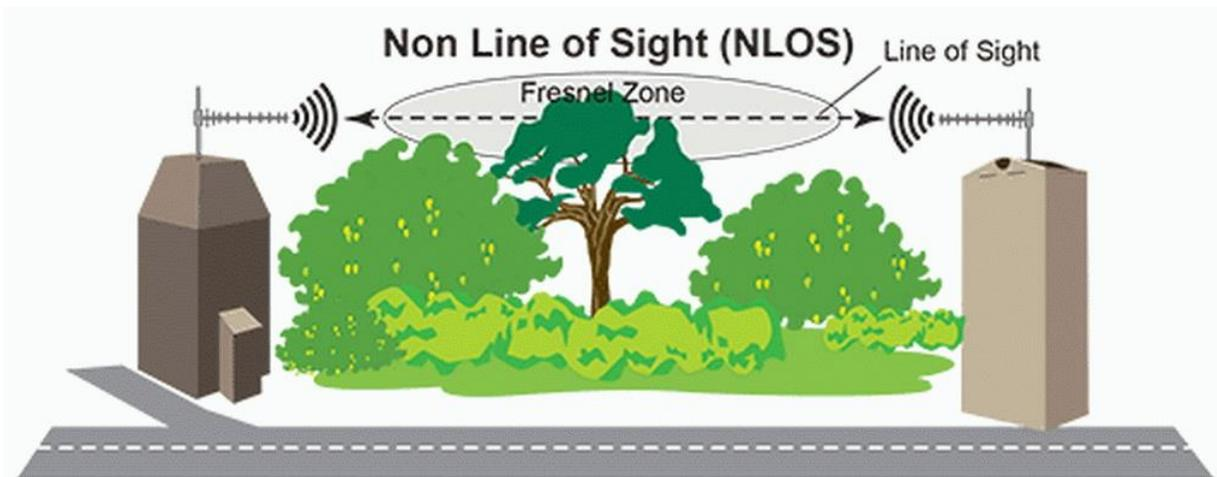
Near Line Of Sight can usually be dealt with using better antennas, but Non Line Of Sight usually requires alternative paths or multipath propagation methods.
