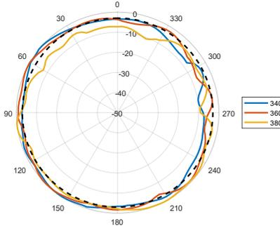
Elevation1 (Side View): 410–470 MHz
