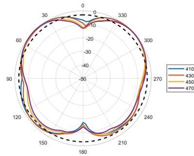
Elevation2 (Side View): 698–960 MHz
