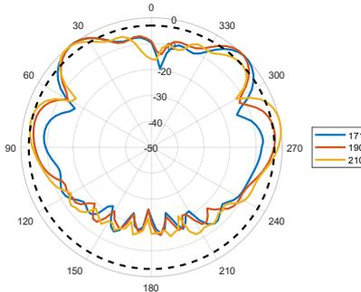
Elevation1 (Side View): 2300–2700 MHz
