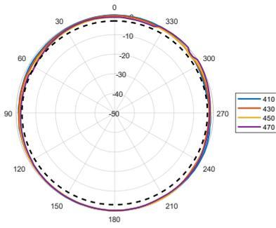
Azimuth (Top View): 698–960 MHz
