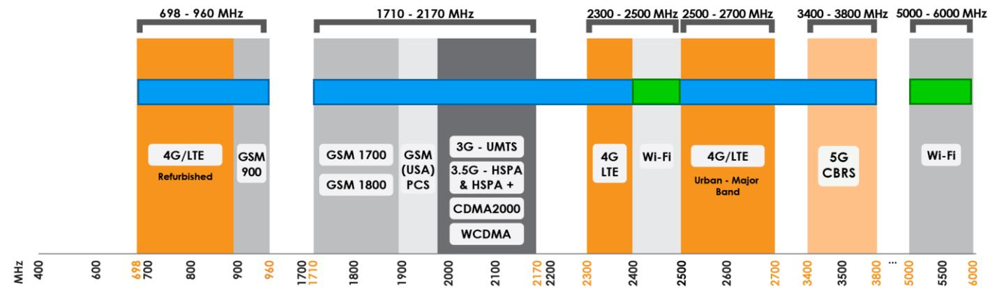
Indicates the 5G/LTE bands on which PUCK-5 works       Indicates the Wi-Fi bands on which PUCK-5 works
