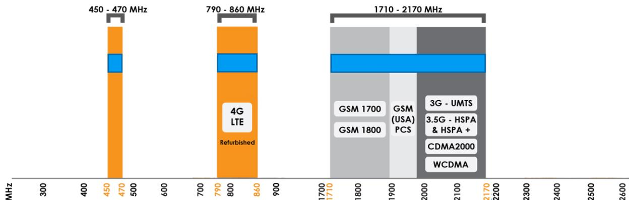
Indicates the LTE bands on which XPOL-16 works
