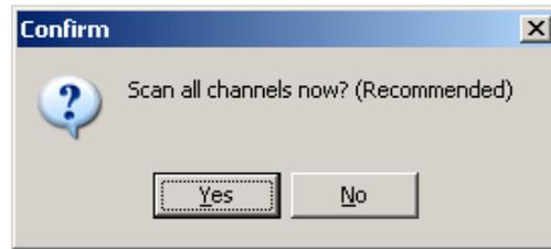
All channels are checked and the program suggests to automatically selecting the best channel by pressing "Yes".
