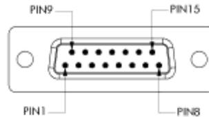
**Table 4.2. NMS 15-PIN FEMALE D CONNECTOR PINOUT**
