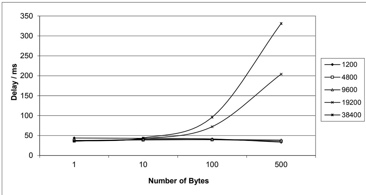
**18.2.2 Transmission delays - 12.5 kHz channel, FEC ON, no NMS**
