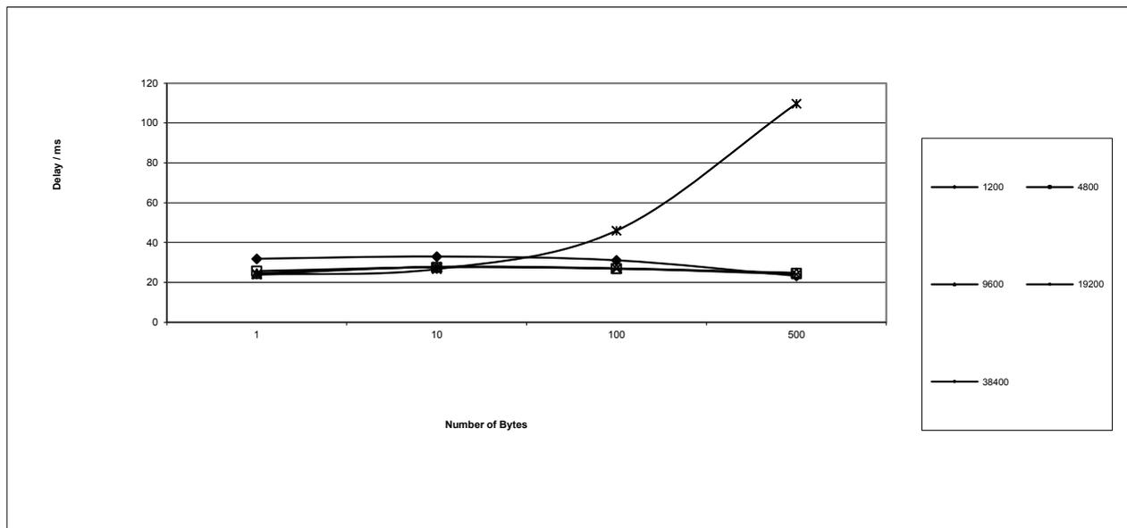
**18.2.4 Transmission delays - 25 kHz channel, FEC ON, no NMS**
