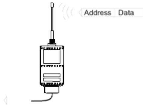
Reception addressing has been set ON, but both the primary and secondary RX addresses of the radio modem are different from the address of the received data packet.
