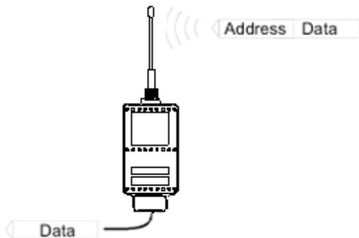
Reception addressing has been set ON and either the primary or secondary RX address of the radio modem is identical to the address of the received data packet.
