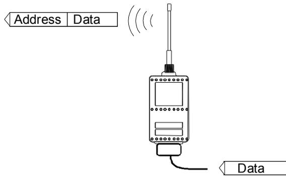
Transmission addressing has been set ON. The radio modem will add the primary TX address to the beginning of the data packet.
