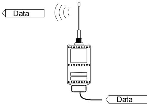
Transmission address has been set OFF. Radio modem will transmit the data packet as such.
