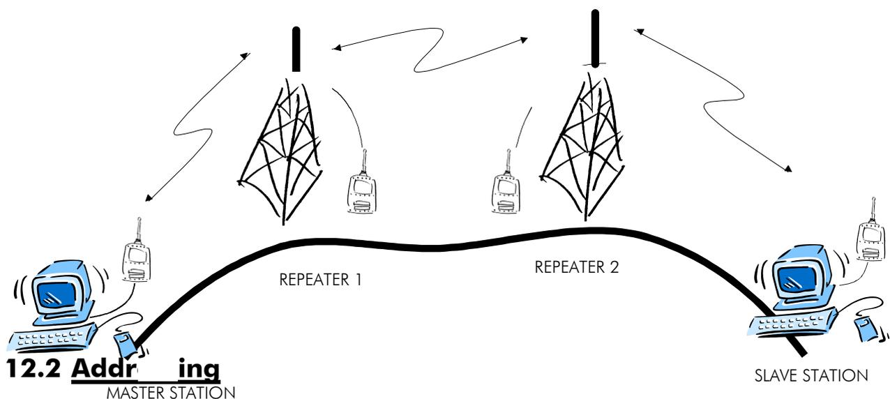
Addresses can be used to route a data message to the desired destination or to separate two parallel networks from each other. In networks with repeaters it is usually necessary to use addresses to prevent data messages from ending up in loops formed by repeaters. In case of setting the "Message Routing" function in use, Tx / Rx addresses are ignored by the modem.
