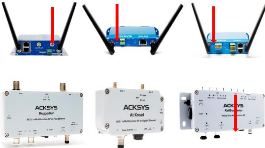
Ex: For some routers like RuggedAir, a RESET button is accessible by opening the cover.
