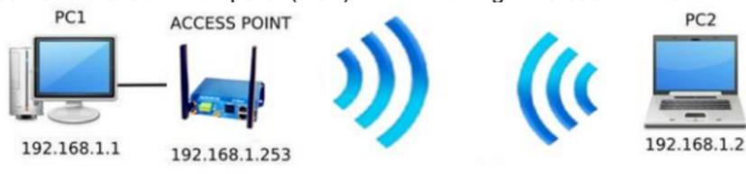
Set up the PC2 Wireless network interface according to the default parameters of the ACKSYS AP device (802.11gn, SSID "acksys", no security, static IP 192.168.1.253/24).
