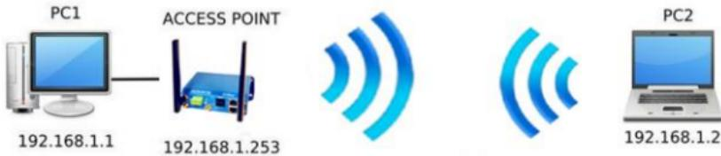
Set up the PC2 Wireless network interface according to the default parameters of the ACKSYS AP device (802.11gn, SSID "acksys", no security, static IP 192.168.1.253/24).
