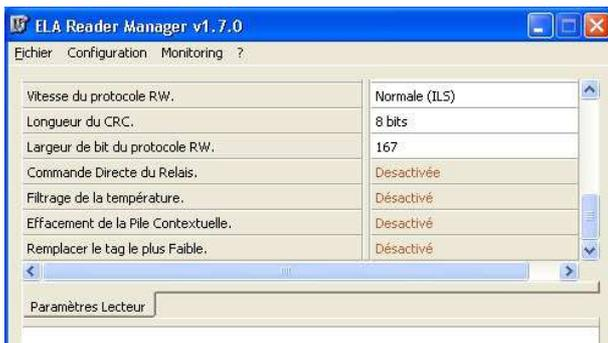
According to the reader's firmware version, some settings can be deactivated and their fields are displayed as greyed fields. The firmware's update is not required except if these settings are required for the application.
